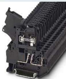
6.3 A, lever-type fuse terminal block for 5 x 20 mm cartridge fuses
