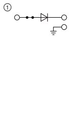
0.5 A, diode terminal block, 1N 4007 (1300 V/0.5 A), conducting direction: from left to right
