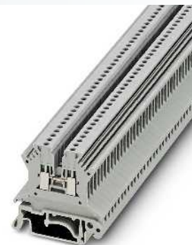
1.5 (1.5) mm 2 , 17.5 A, feed-through terminal block
