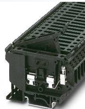
4 (4) mm 2 , 6.3 A, lever-type fuse terminal block for 5 x 20 mm cartridge fuses
