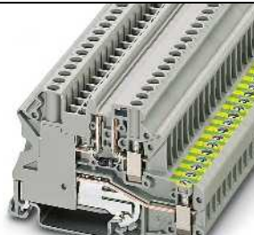
0.5 A, diode terminal block, 1N 4007 (1300 V/0.5 A), conducting direction: from left to right
