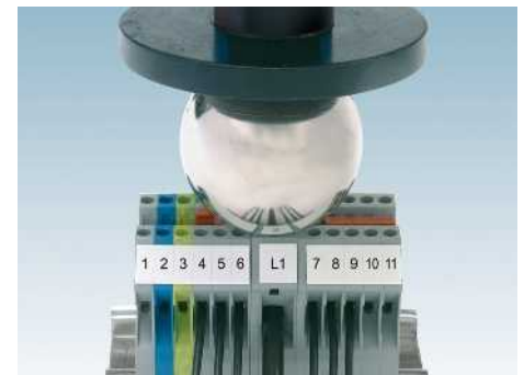
Back of hand safety Test ball with 50 mm diameter
